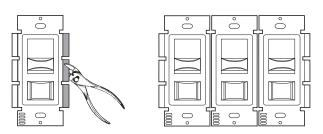
Never install low and high voltage wiring in the same wall box. A physical divider must exist when ganging low voltage and high voltage controls.
